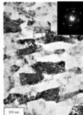
Figure 3. Microstructure of the 6063 alloy after the direct extrusion combined with ECAP-PC
